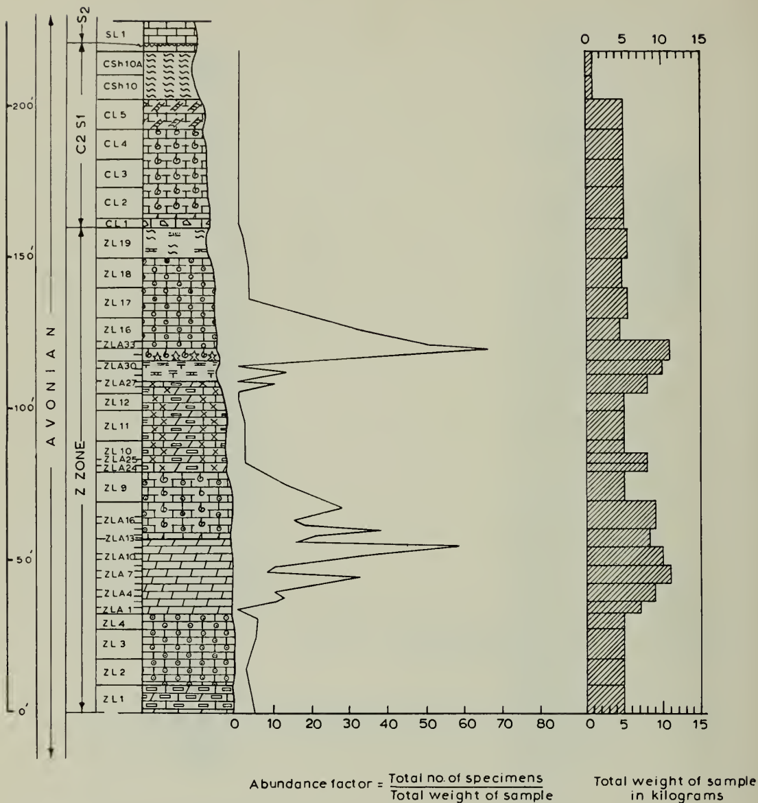
FIG. 71. Lithological section of the Z and S 2 Zones of the North Crop of the South Wales Coalfield showing the abundance factor of conodonts in each sample, and the total weight of limestone dissolved. For details of collecting localities see Fig. 7 and also p. 25.
